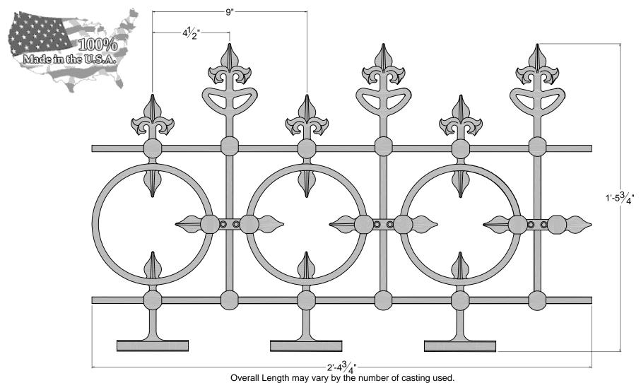
Primary castings (AIC-635, 636) are joined by a pair of  $\frac{3}{8}$ " round bars and a spacer casting (AIC-637).
