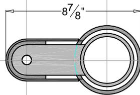
Detail: Bollard & Receiver Plan at locking interface
