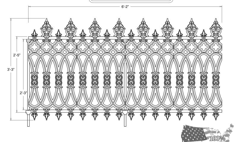
This fence section is composed of 2 castings:
