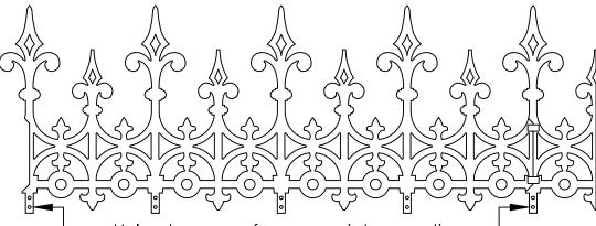
Holes shown are for appropriate mounting brackets. Flat roof and standard angle roof brackets are included at no extra charge.
